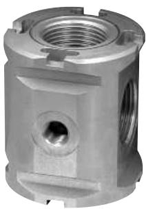
P3Y Series Manifolds provide up to 4 extra outlet ports. They may be assembled at any position in a combination e.g. before the lubricator to provide oil free take off or at the end of a combination to provide extra outlet ports.
