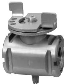
Ball / Lockout Valve shuts off downstream line pressure in the closed position with a 90° turn of the handle. In the closed position, inlet air pressure is blocked and downstream / system air is exhausted through a threaded port. To prevent unauthorized adjustment, the padlock slide may be assembled on either side. It is recommended that this slide is installed after final system assembly.
