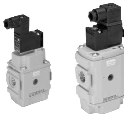
Remotely operated dump valves automatically shut off upstream pressure and exhaust the downstream pressure when the pilot pressure is released.
